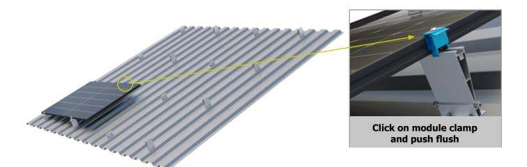
Now slide the next module under the mid clamp, adjust the mid clamp to the module frame height and tighten the screw (tightening torque 8-10 Nm).
