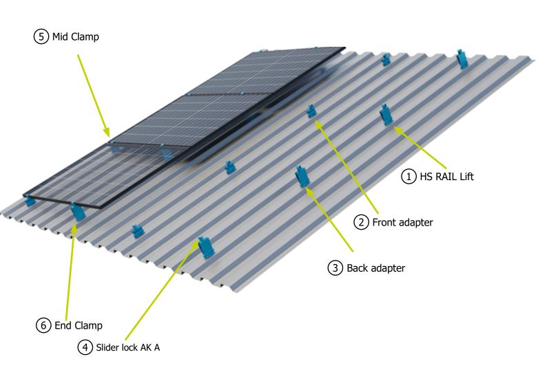
Note: On the following pages, module installation is shown vertical. The module is mounted horizontally according to the same scheme. This requires the module clamps on the short sides to be released.
