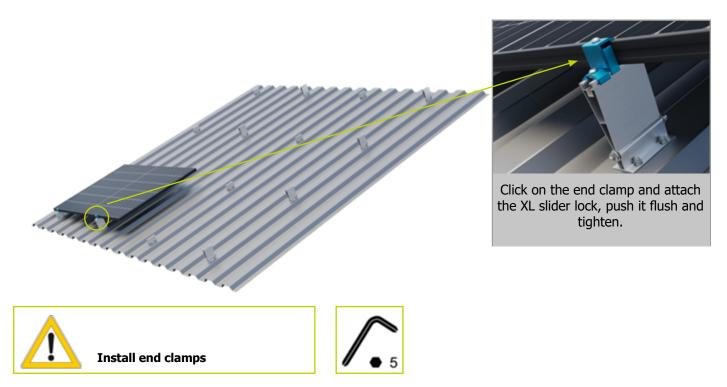
Ensure that the end clamp clamps the module frame with the clamping surface defined by the module manufacturer. Install the slider lock XL on the back adapters at the end of the module field.
